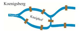
To solve this problem, Euler built a graph G whose vertices are the different adjacent regions, if there were no bridge, and where each edge represents a link between two regions via a bridge. In order for a pedestrian to cross each bridge exactly once, G must contain a Eulerian cycle, which is not the case because G contains four vertices of an odd degree.
