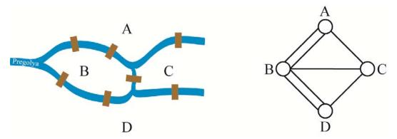
When all the vertices in a graph are of an even degree it is easy enough to draw a Eulerian cycle. We can do this as follows, for instance.
