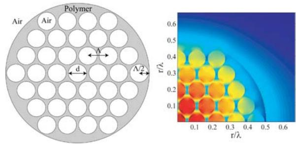
Fig. 5. Highly porous microstructured optical fibers for low loss guiding of THz light. Light is confined predominantly in the air holes.
