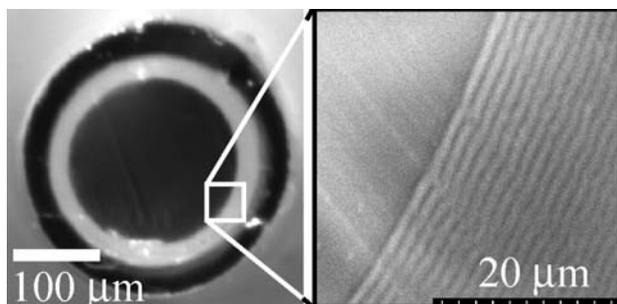
Fig. 1. Example of a plastic photonic bandgap Bragg fiber containing 100s of PMMA/PS layers.
