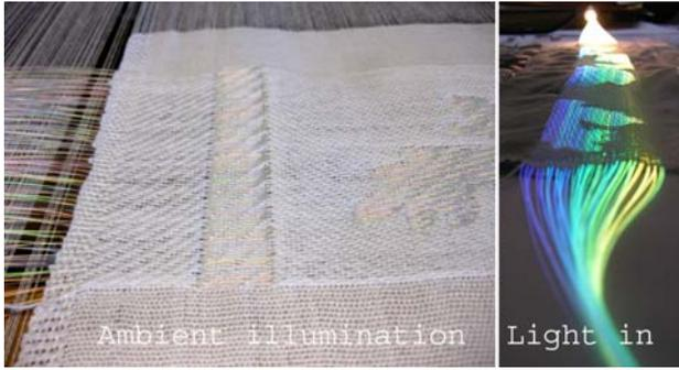
Fig. 3. Photonic bandgap textiles under ambient illumination and with light launched into it.
