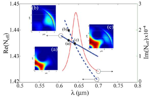
Fig. 8. Dispersion relations of a core guided mode (thick solid line) and a surface plasmon (thick dashed line) in the vicinity of phase matching.
