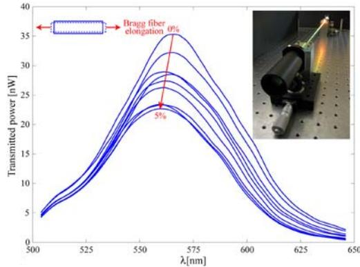
Fig. 4. Transmission peak (color) of a Bragg fiber can be shifted by fiber elongation.
