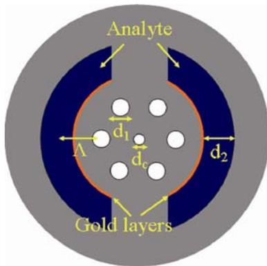
Fig. 7. Plasmonic sensor using metallized microstructured fiber. Central region is a core of a single mode waveguide. On the periphery one finds a metallized air channel filled with analyte.
