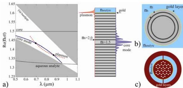
Fig. 9. Schematics of various photonic crystal waveguide-based SPR sensor implementations. a) Single mode planar photonic crystal waveguide-based SPR sensor. The dispersion relation of the core guided mode is in solid blue, that of the plasmon is in thick dashed red. Inset - coupler schematic;  $|S_z|$  of a plasmon (left) and a core mode (right). b) Solid core Bragg fiber-based SPR sensor. c) Microstructured core, honeycomb photonic crystal fiber-based SPR sensor.
