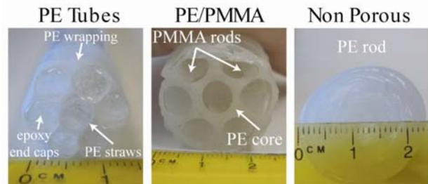
Fig. 6. Porous microstructured optical fiber preforms made by PE tube stacking, PE molding in a PMMA mold, and, finally, molding of a rod fiber preform in a Teflon tube.
