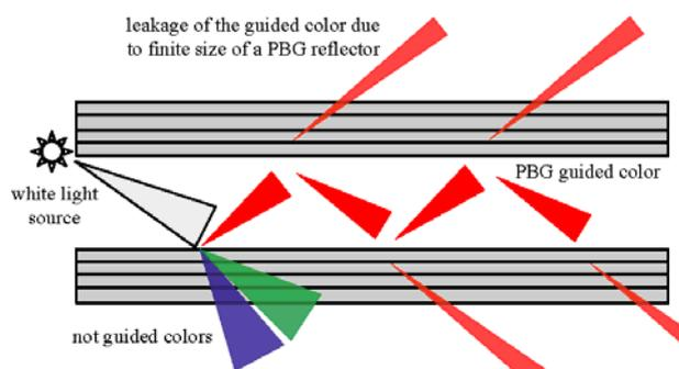
Fig. 2. Light emitting Bragg fiber does not require mechanical perturbations for light extraction.
