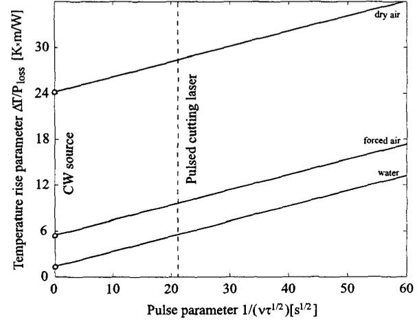
Fig. 2. Temperature rise parameter curves as a function of a laser pulse parameter,  $\nu$  - pulse repetition rate,  $\tau$  - pulse duration. Different curves correspond to the different cooling mechanisms.
