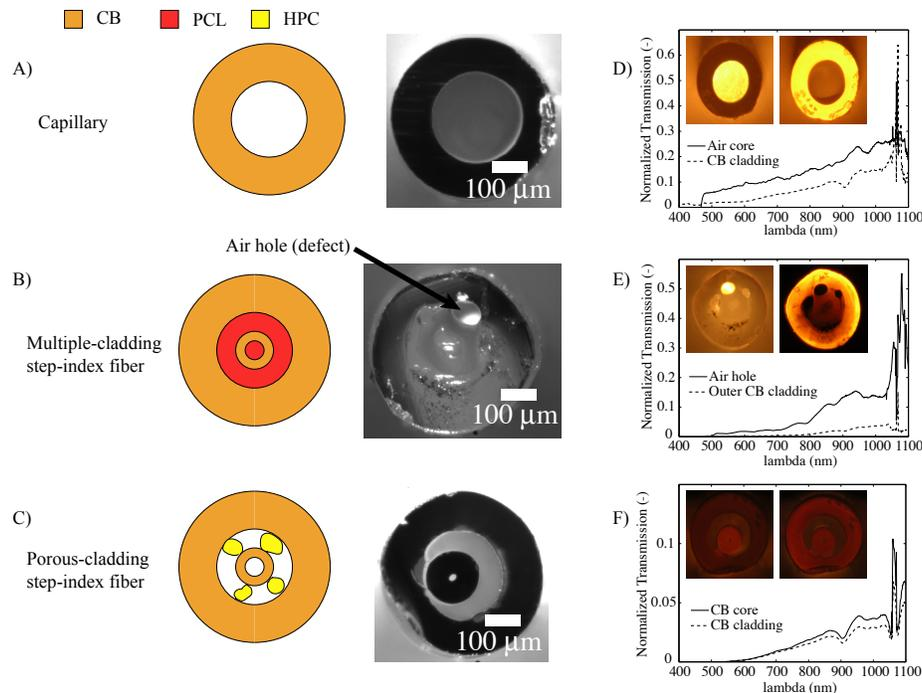
Fig. 1. (A)-(C) Schematics of the preform geometries and microscope images of the drawn fiber cross-sections using various fabrication strategies. (D)-(F) Transmission spectra of the biodegradable optical fibers with images of the transmitted light as insets. The lengths of the measured segments are 6.95, 3.25, and 8.05 cm respectively.
