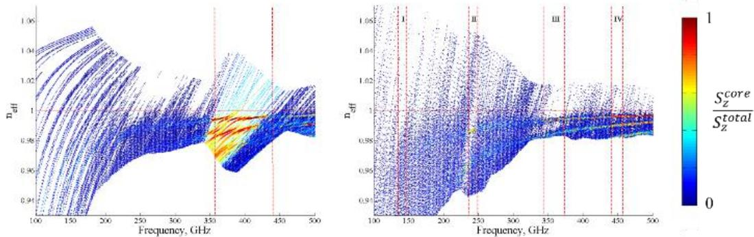
Fig. 2 Band diagrams of (a) the waveguide with numerically optimized reflector structure and (b) the fabricated waveguide with the bridge thickness of  $\sim 200\mu\text{m}$ .
