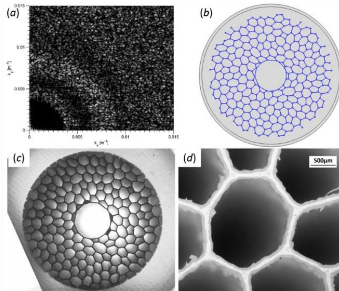
Fig. 1. (a) Hyperuniform point pattern in k-space. (b) Waveguide and a simulation cell used in our numerical calculation. (c) The fabricated waveguide with the bridge thickness of 200µm in the cladding. (d) Zoom of the reflector region shown in (c)
