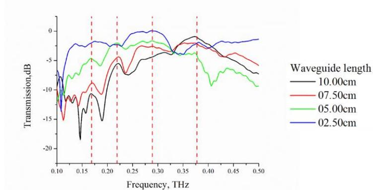
Fig. 3 The transmission spectrum of the fabricated waveguides with bridge thickness of  $200\mu\text{m}$
