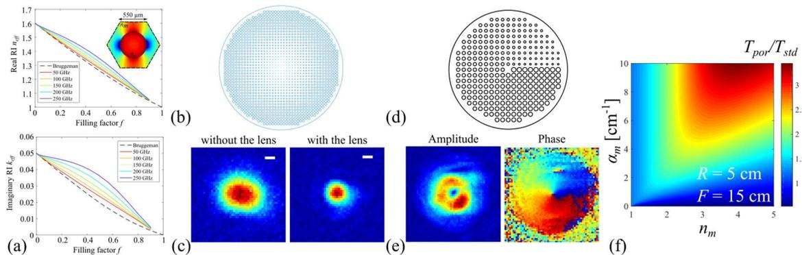
Fig. 1. (a) Effective refractive index when varying the hole size. (b) Porous lens. (c) THz imaging at 200 GHz with and without the lens. (d) Design of the OAM phase plate. (e) Amplitude and phase of the obtained OAM state. (f) Transmission ratio as a function of the absorption losses and refractive index
