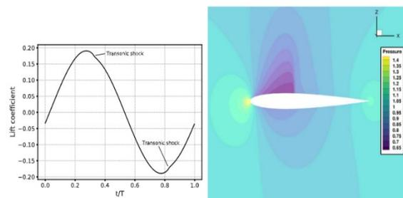
Figure 1: Lift coefficient prediction using the Vortex Lattice method (credit: Parenteau & Laurendeau, 2021)
