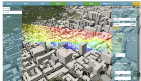
Figure 1: interactive visualization of urban microclimate simulation from the CityFFD engine (credit: Mortezaazadeh et al., 2022)
