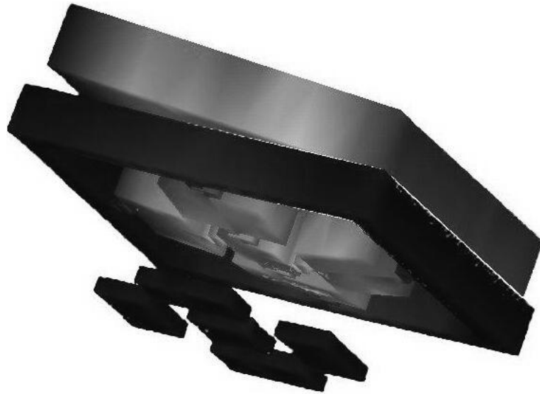
Figure 9: Simulation of tilt in an individual mirror of the adaptive optics array, The 5 stationary electrodes under the actuator layer enables piston motion and tilt on two axes.
