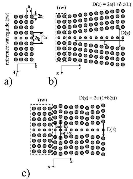
FIG. 1. (a) Dielectric profile of a reference 2D photonic crystal waveguide as formed in a square array of dielectric poles in air by a linear sequence of somewhat smaller dielectric poles. (b) Linear taper in a photonic crystal with "unzipping" photonic mirror. (c) Stochastic variations in a waveguide core size along the direction of propagation.
