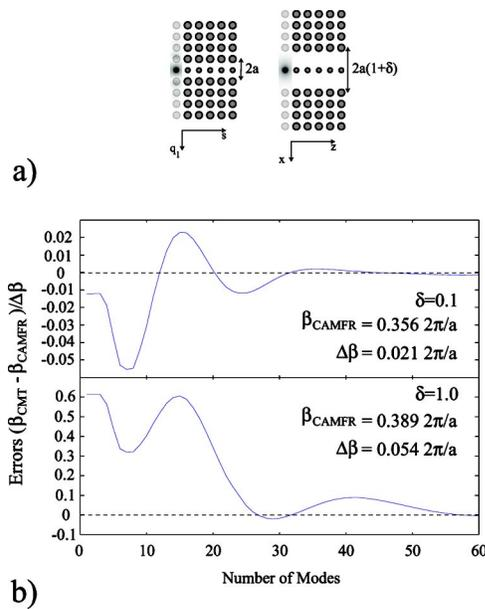
FIG. 3. (a) Schematics of a reference waveguide (left) and a perturbed uniform waveguide (right) of a larger core. Electric energy distributions in the fundamental modes are presented in the corresponding first unit cells. (b) Convergence of the fundamental mode propagation constant for a weakly  $\delta=0.1$  and a strongly  $\delta=1.0$  perturbed reference waveguide in a CMT framework.
