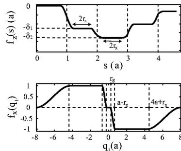
FIG. 2. Auxiliary functions for the coordinate mapping of a reference 2D photonic crystal waveguide [Fig. 1(a)] onto a waveguide of a changing core size [Fig. 1(c)].
