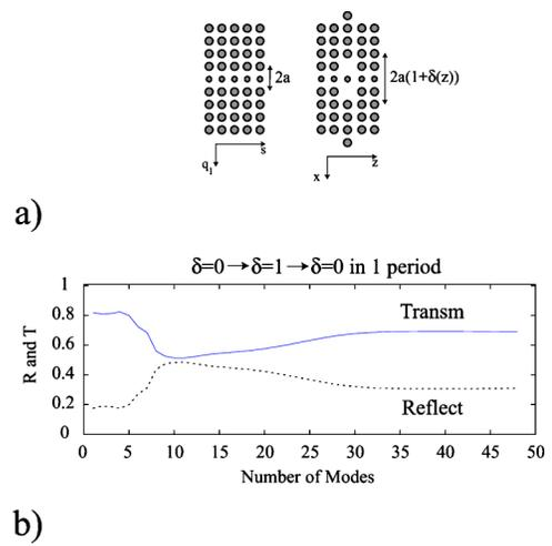
FIG. 4. (a) Schematics of a reference waveguide (left) and a single-cell defect in a reference waveguide (right). (b) Convergence of the transmitted and reflected powers into the forward and backward propagating fundamental modes as calculated by CMT and  $\delta=1.0$  perturbation.
