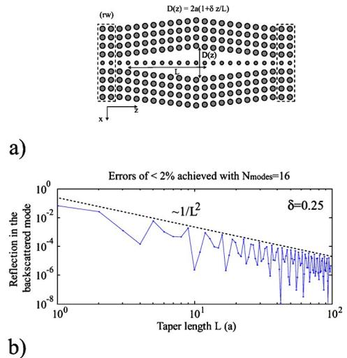
FIG. 5. (a) Taper of an “unzipping” reflector around an index guiding waveguide. To the left and to the right of the taper the photonic crystal waveguide is infinite and is described by the first unit cell of the schematic. (b) Reflected power from the taper at  $\omega=0.25 \times 2\pi c/a$  as a function of taper length  $L$ . Observe a  $1/L^2$  decrease of the reflected power with taper length.
