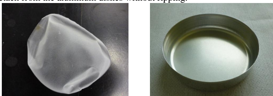
Fig. 8. PEO films with different concentration of Li-salt: a) 1:20 \text{Li}^+ /PEO ratio results in highly crystalline opaque films, b) 1:5 \text{Li}^+ /PEO results in jelly-like transparent films.
