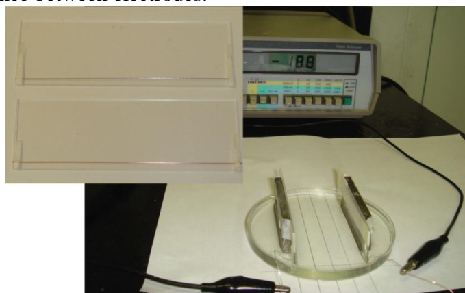
Fig. 2. Setup for measuring the short-circuit currents and the open voltages of an Al-NaOCl galvanic cell. The inset shows two glass plates to which the copper and the aluminum wires are attached.
