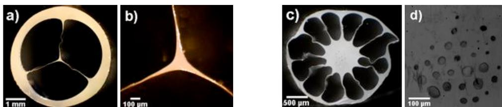
Fig. 1. (a) Cross section of the suspended core fiber  $\Phi_{\text{fiber}} = 5 \text{ mm}$ , and (b) close-up view of the suspended core region ( $\Phi_{\text{core}} = 150 \mu\text{m}$ ). (c) Cross section of the porous core fiber  $\Phi_{\text{fiber}} = 3 \text{ mm}$ , and (d) close-up view of the suspended porous core ( $\Phi_{\text{core}} = 900 \mu\text{m}$ )
