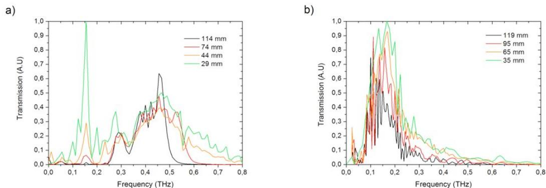
Fig. 2. Normalized transmission as a function of frequency between 0.01 and 0.80 THz for (a) the suspended solid core fiber, and (b) the suspended porous core fiber.
