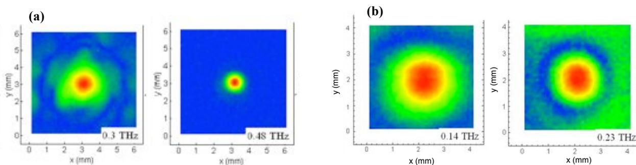
Fig. 3. Near field imaging of the output field profile of (a) suspended solid core fiber at 0.30 and 0.48 THz, and (b) suspended porous core fiber at 0.14 and 0.23 THz.
