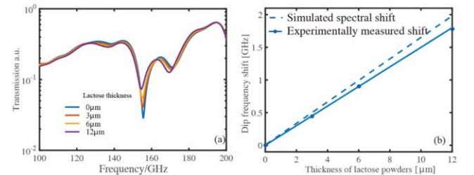
Fig. 3 (a) Measured transmission spectra of the THz Bragg waveguide (with a  $300\mu\text{m}$  defect), when different amounts of lactose powders are loaded into the core. (b) Experimental and theoretical spectral shift of the transmission dip found at the right edge of the bandgap as a function of the layer thickness.
