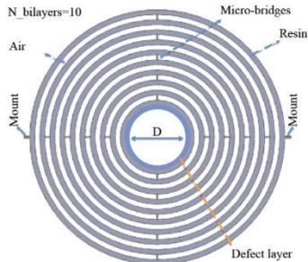
Fig. 1 Schematic of the designed Bragg fiber with a defect layer.
