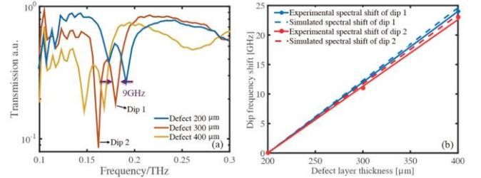
Fig. 2. (a) Measured transmission spectra of the THz Bragg waveguide featuring a defect layer of different thicknesses. (b) Experimental and theoretical spectral shifts of the two transmission dips as a function of the defect layer thickness.
